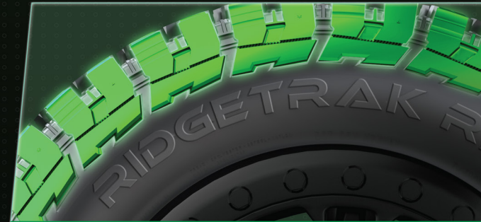
Aggressive sidewall lugs increase durability and grip
